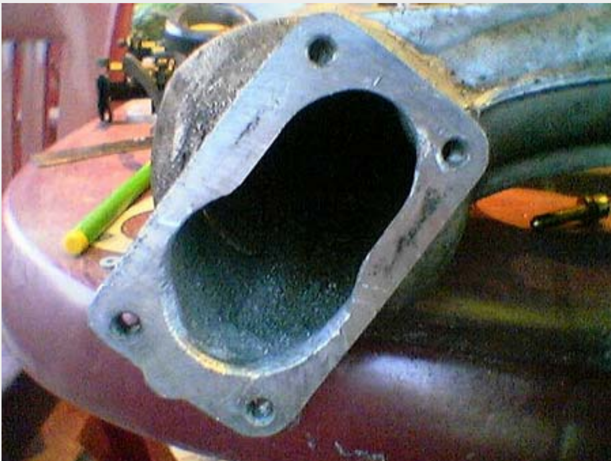
This is the bored opening nearly to size.
