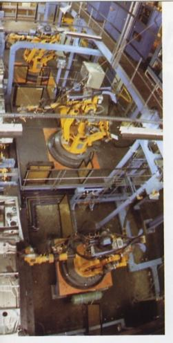
Because the car is immersed totally in a giant bath that uses electric polarity to reach places that just aren't accessible by spraying or other means.
