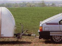
Citroën's unique self-levelling suspension. Lower the car's height to make disconnecting the trailer easier. Then simply raise it afterwards.
